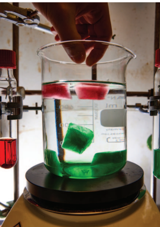
Illustrative experiment: the red cubes made of moulded water ice float to the top normally; the green cubes of heavy water sink.
