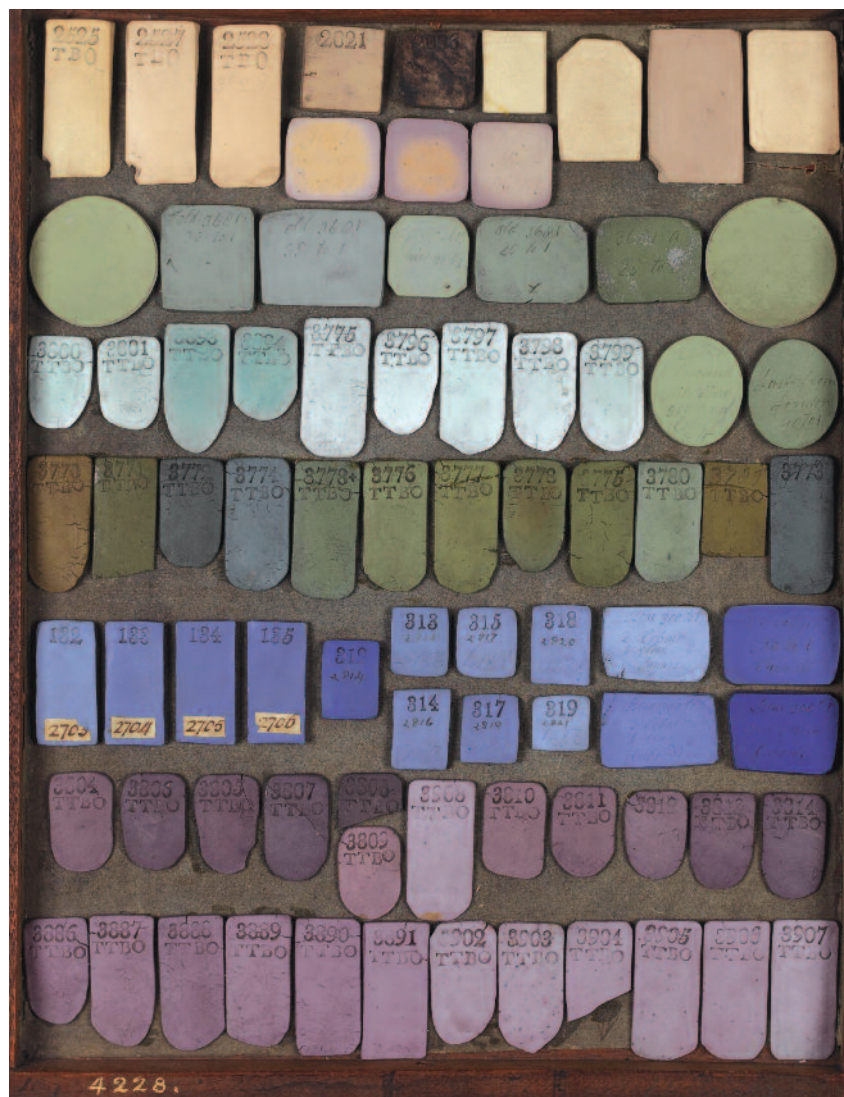
Tray of Jasper trials, 1773. Each trial piece is marked with a number that corresponds to an entry in Wedgwood's 'Experiment Book'. Many pieces are impressed with the firing instructions, for example 'TTBO' for 'tip-top of biscuit oven'.
