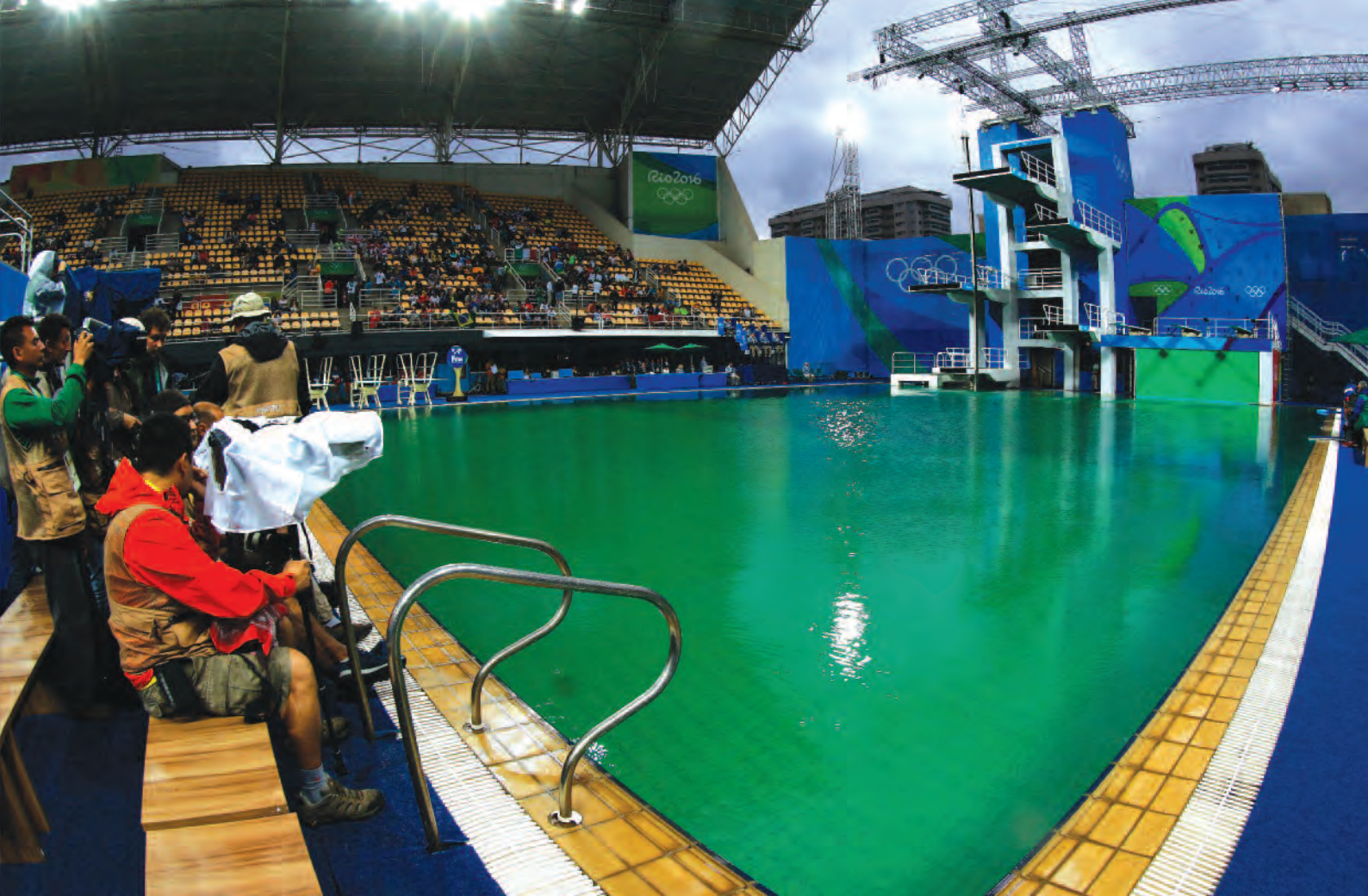
The water of the Rio Olympic diving pool turned green after 80 litres of hydrogen peroxide was mistakenly added to the pool during cleaning. The hydrogen peroxide neutralised the chlorine and allowed algae to bloom. Fernando Frazão/Agência Brasil/CC-BY-2.0
